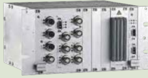
Trainnet® Ethernet Switch (functions: switch with PoE)
