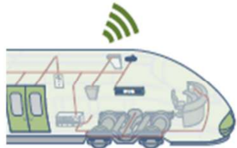
Figure 1. Schematic drawing of measurement equipment installed on a bogie
