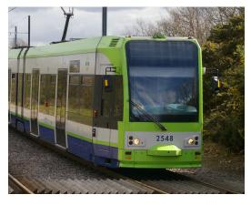
The EKE-Trainnet<sup>®</sup> Physical Prevention of Over-Speeding (PPOS) system prevents trams from overspeeding. It allows the operator to set speed limits over the whole network by using trackside beacons and/or Global Navigation Satellite System (GNSS) together with distance measuring. The PPOS reads the speed limits from balises positioned on the tram tracks. If a tram is over-speeding, the system automatically applies service brakes, stops the tram and sends an alarm to the Control room.
