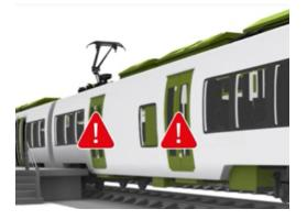
The EKE-Trainnet<sup>®</sup> Automatic Selective Door Operation (ASDO) is developed to improve passenger operation at stations where the platforms are shorter than the trains. ASDO enables an automatic check of the train's position and the platform configuration so only the doors that can be safely opened are released. Passenger comfort and safety is enhanced while allowing for shorter stops at stations.
