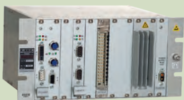
VCU with CAN and Digital Input/Output Interfaces
