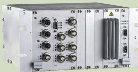
Trainnet® Ethernet Switch (functions: switch with PoE)
