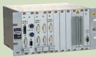
WTB-Ethernet-CAN- Serial Links Gateway
