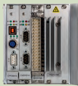
Version with CAN interface module and extra logging memory
